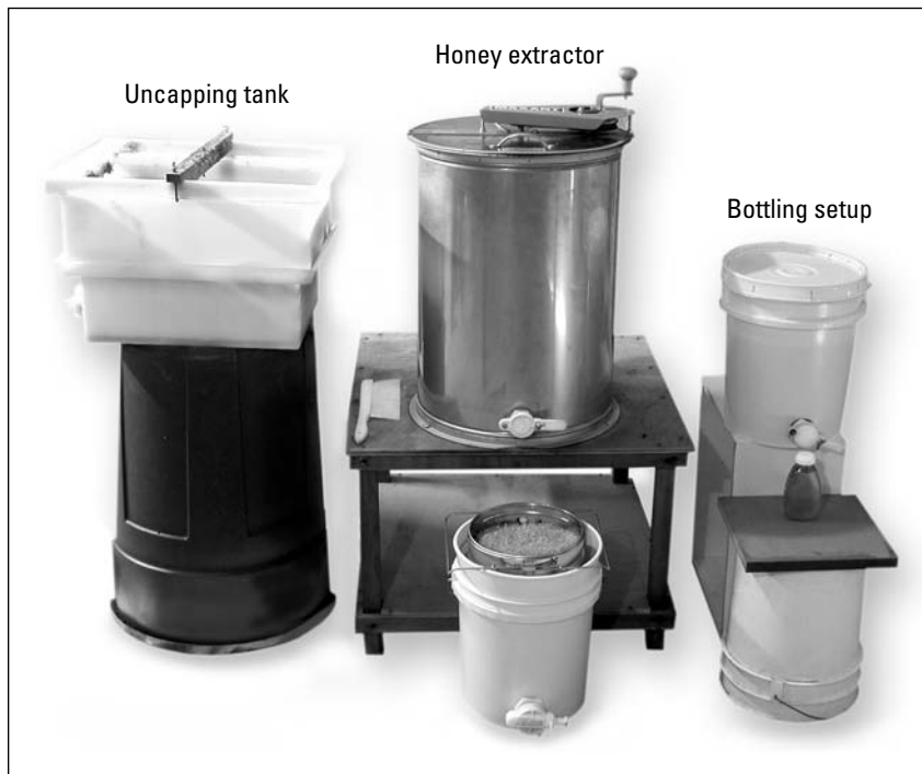
Figure 14-8: Here's the setup, left to right, in my garage for extracting honey.
